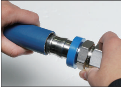
2. Cover first barb of end connection with hose. (Lubrication fitting stem with light oil may ease assembly)
