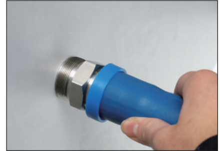
3. Hold end connection against flat surface, Grip hose and push with a steady force until hose seats into blue finishing.
